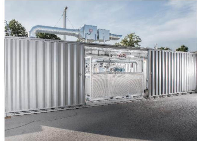
150 kW SOEC unit in Dresden, Germany
